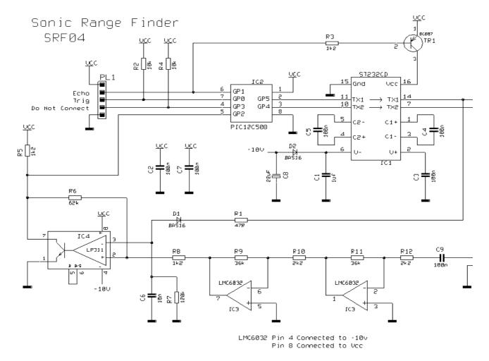
The circuit is designed to be low cost. It uses a PIC12C508 to perform the control functions and
