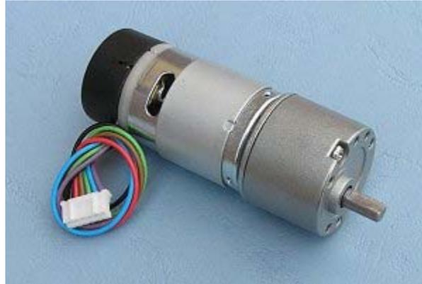
The EGM30 (encoder, motor, gearbox 30:1) is a 12v motor fully equipped with encoders and a 30:1 reduction gearbox. It is ideal for small or medium robotic applications, providing cost effective drive and feedback for the user. It also includes a standard noise suppression capacitor across the motor windings.
