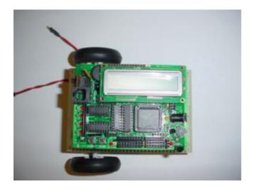
Insert the motor connectors to Handyboard motor driver ports (i.e. Port 2 and Port 3).
