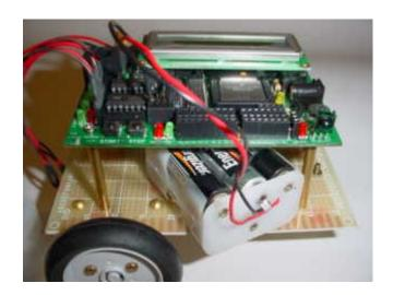
Put the 8 x AA battery on Handyboard power supply holder.
