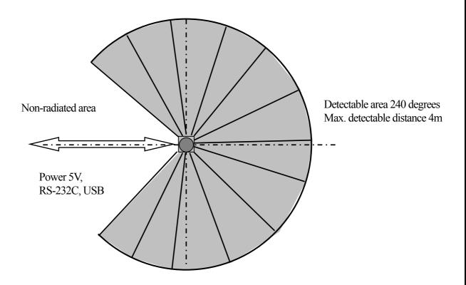
Note) The above figure shows the detectable area by detecting object with 70mm x 70mm. Max. detecting distance is changed depending on a kind of detecting objects.
